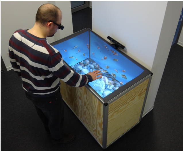
Figure 2: Photo taken of our touch-enabled prototype (the perspective was registered with the camera for the photo).
