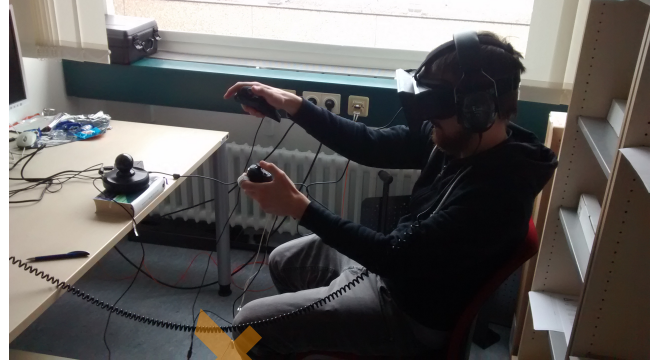
Figure 1: Participant during an experimental session Participants wore head-mounted display, circumaural headphones and held in both hands the Razer Hydra's controllers. Galvanic skin response sensors were wrapped to their fingers
