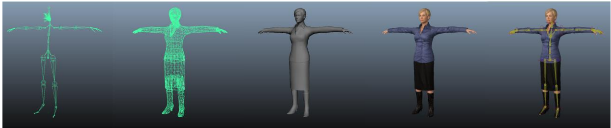
Figure 2. Avatar components. From left to right: skeleton, mesh, surface, texture, control rig.
