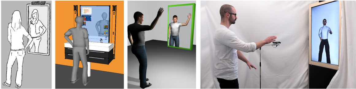
Figure 1: Left three images: Sketches through the design phase of the fake mirror system. Second from left depicts a potential application in a real living scenario. Right image: Actual implementation of the system and setup for typical studies on avatar embodiment. Note that the mirrored avatar looks perspectively correct for the user and is distorted in this picture due to the applied stereoscopy and head-tracking.
