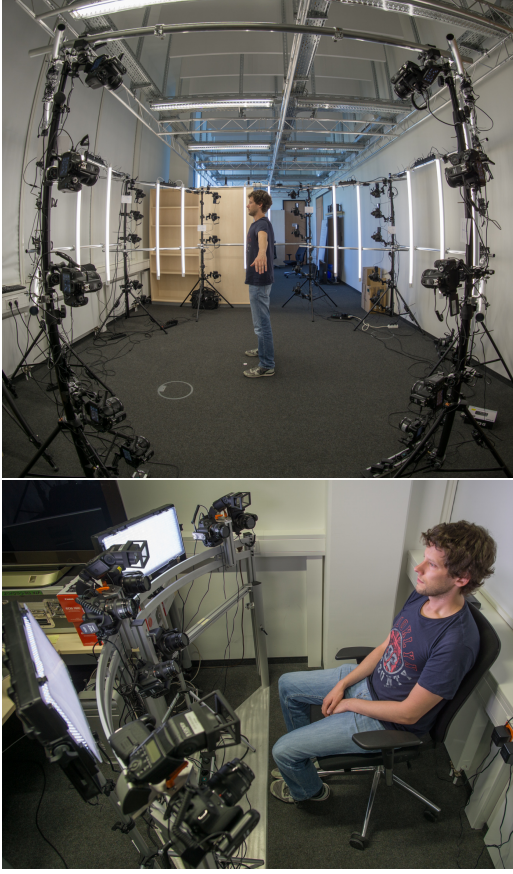
Figure 2: Our custom-built full-body scanner (left) and face scanner (right) are both based on multi-view stereo and consist of 40 and 8 DSLR cameras, respectively.
