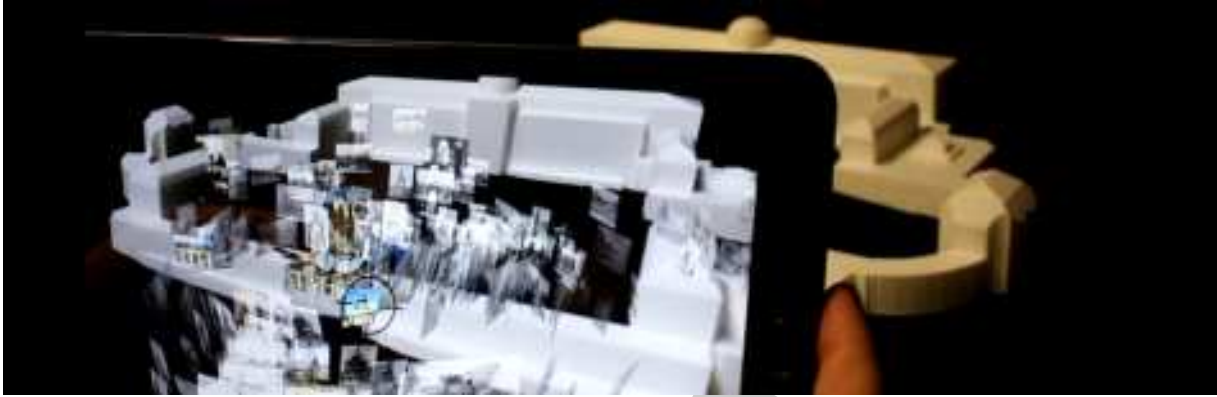
Figure 1: Hand-held Augmented Reality for spatial browsing of photographs registered to physical model
