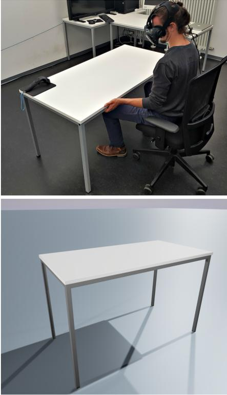
Figure 1: General overview of the experimental design. Top: The participant is seated in an office chair before a real physical table while wearing a head-mounted display. Bottom: In the virtual environment the physical table is substituted by a virtual replica of the real table. During the study, the spatial alignment between the real and the virtual table and hence the coherence between the real physical and the virtual world are modified.
