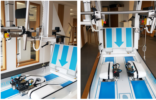
Figure 2: Example of a gait robot used for clinical rehabilitation. Gait robots typically apply a cyclic movement that needs to be supported by the patients own gait force.
