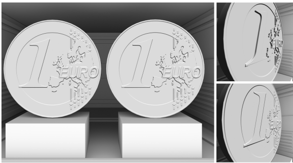
Figure 2: Left: Side by side comparison of 2 coins as seen in each trial. Right: Oblique view of both coins to emphasize the differences. Top right: Geometry reference coin with a minting of 5 mm. Bottom right: Corresponding flat coin with applied normal map.
