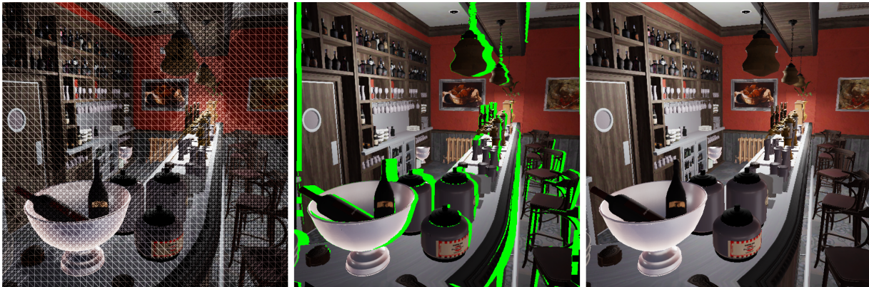
Figure 1: The proposed hybrid rendering system reprojects the source image of the left viewpoint into the right viewpoint by using an adaptive 3D grid warping approach (left), detects disoccluded regions (middle, marked in green) and resolves them correctly through adaptive real-time ray-tracing (right).
