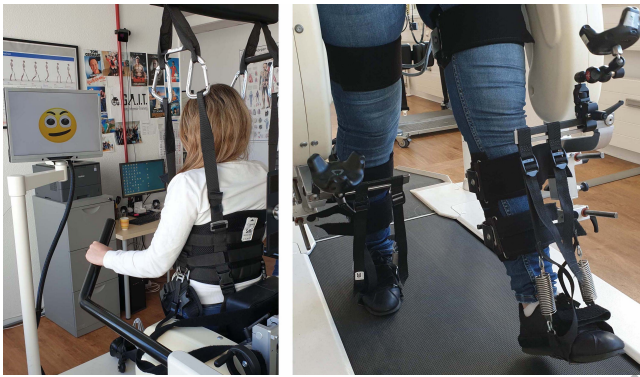
Figure 4: Setup. The visual feedback presented in the physical scenario (left). Two motion trackers attached to gait orthosis (right).
