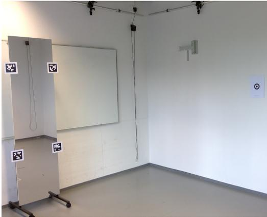
**Figure 4: Laboratory setup: Mirror with Apriltag markers (left), calibration marker (right), each 1.40 m distance from participant.**
