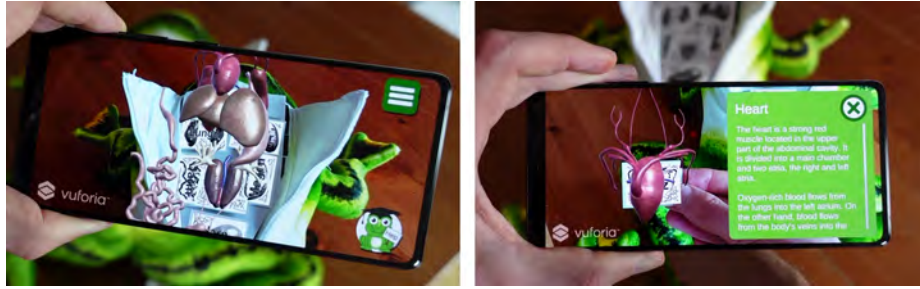
Fig. 1. When detecting the markers with a smartphone, Horst-TAR displays 3D models of the organs. Touching the organ reveals biological information.
