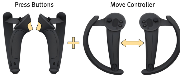
Figure C3.4: Sketch of the body weight modification interaction through gestures. Participants had to press the trigger buttons on each controller and move the controllers either apart (increase body weight) or together (decrease body weight).
