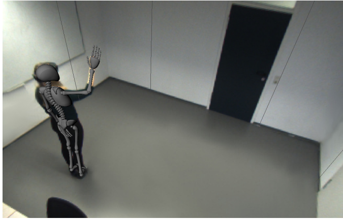
Figure C4.2: The screenshot of Captury Live’s tracking view shows the user from Figure C4.1 inside our laboratory currently waving to her holographic reflection while her pose is tracked in real-time.
