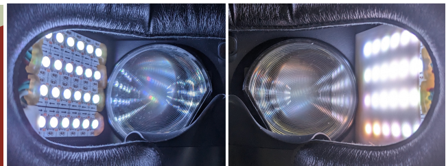
(b) Peripheral Display Extension with 4 x 6 LEDs on each side integrated into the HTC Vive Pro.
