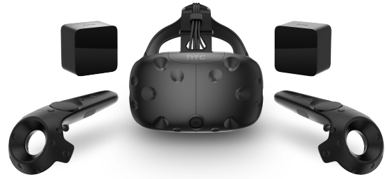
Fig. 1: HTC Vive HMD Family containing two controllers in the left and right front, a head-mount-display that is mounted to the head of the player and two base stations called Lighthouse
