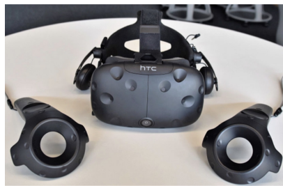
Fig. 1: The HTC Vive is comprised of two input controllers in the left and right front, a head-mounted display (HMD) that is mounted to the head of the player and two base stations called Lighthouses .
