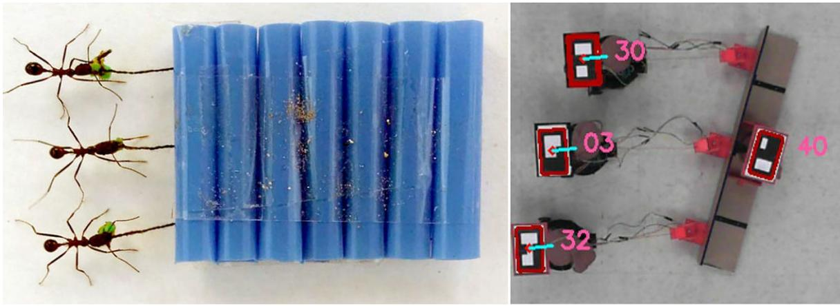
**Figure 10.** Collaboration of multiple robots on the construction sub-task of towing materials, inspired by a collaborative mechanism in social insects [300]; image from [300] and used with license. (Image reprinted from fig. 1 (subfigures *a* and *b*) of the Royal Society Open Science paper of Wilson *et al.* [300], DOI, open access. Used with Creative Commons license CC BY 4.0. Authors holding the image copyright approved the license at publishing.) (Online version in colour.)
