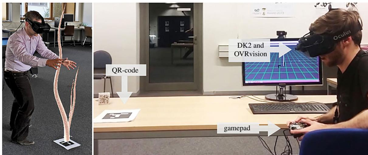
**Figure 11.** Augmented reality interfaces for user interaction with simulations of biohybrid living construction [318]; image from [318] and used with license. (Images reprinted from fig. 8 (subfigures a and b) of the *Frontiers in Robotics and AI* paper of von Mammen *et al.* [318], DOI, open access. Used with Creative Commons license CC BY 4.0. Authors holding the image copyright approved the license at publishing.) (Online version in colour.)
