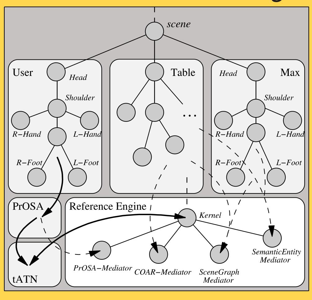
The reference resolution engine (RRE) is embedded in a scene-graph, the basic modelling method for Virtual Reality applications. The ProSA engine and the tATN are analysing and parsing the utterances of the user. During this process the RRE identifies the referenced objects, supported by conceptual short-term memories which are part of the PrOSA engine.
